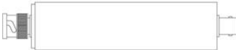
Solar Type 9454-1 High Voltage 40 dB Attenuator
